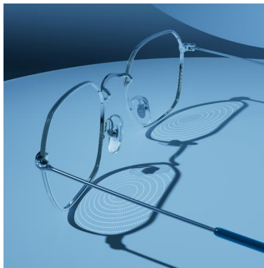
Figure 1: Photograph of the Essilor® Stellest® spectacle lens in a frame, showing the single vision zone (no lenslets) and the zone designed to slow myopia progression using H.A.L.T. technology, which consists of 1,021 lenslets arranged over 11 rings.
