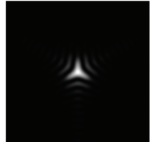
Light source impacted by high-order aberration: trefoil
