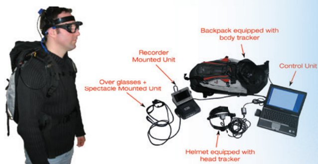
FIGURE 4 The Body Head Eye Movement System (BoHEM) consists of a motion-sensing helmet, backpack, and spectacles. Body and eye movements in response to controlled stimuli are tracked and analyzed, allowing researchers to gain a comprehensive understanding of wearer’s posture and direction of gaze.
